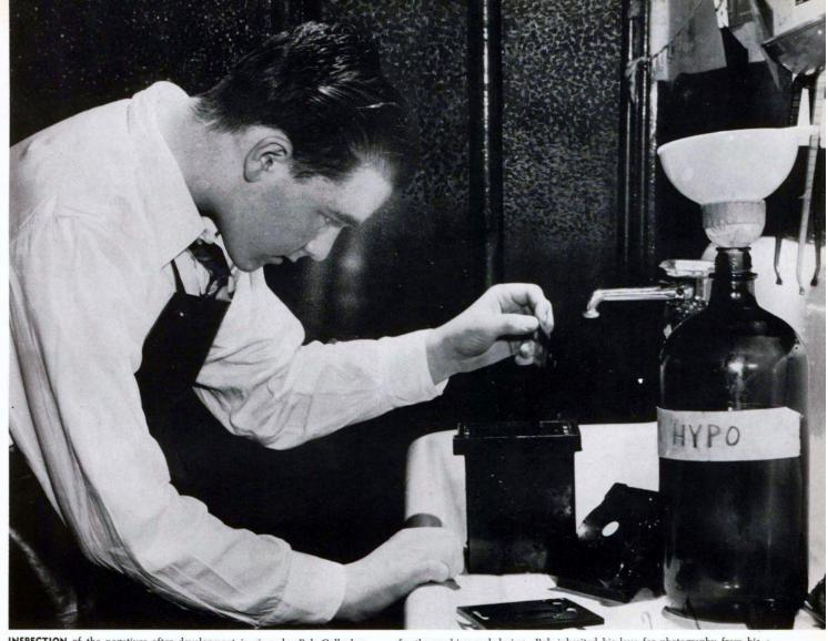
$\label{localization} \textbf{INSPECTION} \ \ \text{of the negatives after development is given by Bob Gallagher.}$  They have just emerged from the acid fixing bath or "hypo", and are ready
